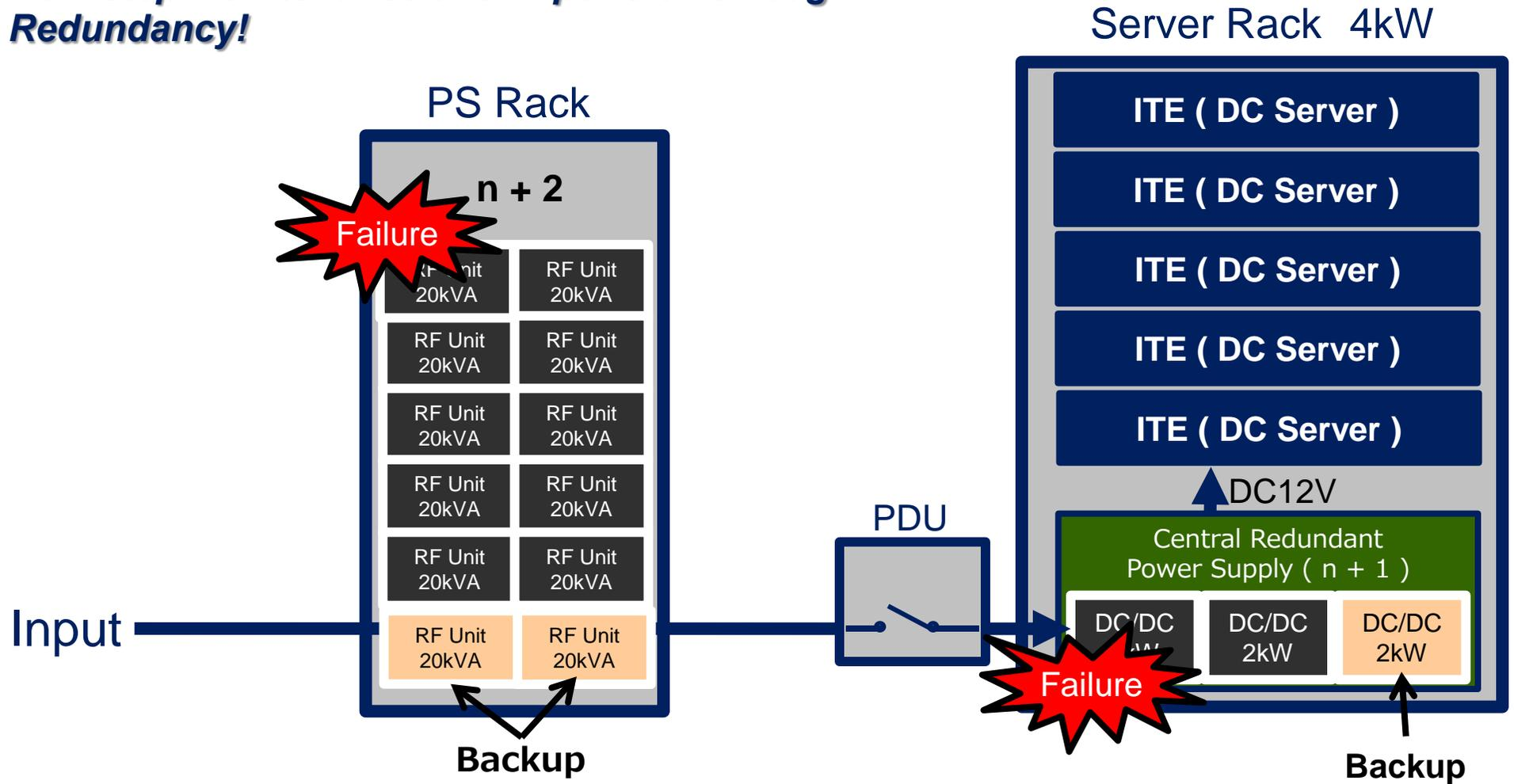
Even if any defect happened on the system, you'll be able to replace all components without any interruption through N+1 redundancy.
